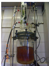
Dual jacket glass 3.5L reactor at AVABIOCHEM
