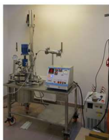
Amar 10L pressure reactor at VTT
