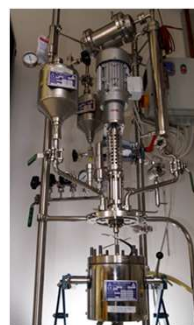
Juchheim 2L bench scale reactor at VTT
